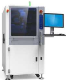
High-speed precision selective conformal coating machine
