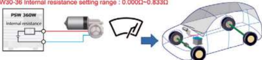
PSW Built-in Resistance Variable Function Simulating Battery Output Resistance and Wire Harness
