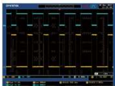
Ch2: Voltage Waveform for Relay 80A for 1s and 0A for 2s
