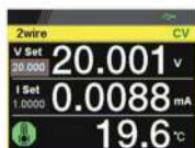
Green: Output Safe is Activated and Output is on with GTL-205A Connected
