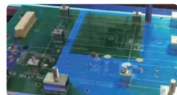
Selective conformal coating of components and IC pins
